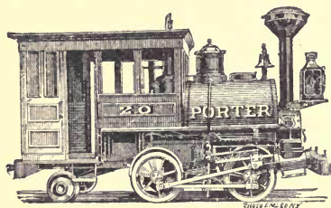
This cut shows cab with side sliding doors and bunker in rear part of cab (filled from outside if for coal) for cold climate.
